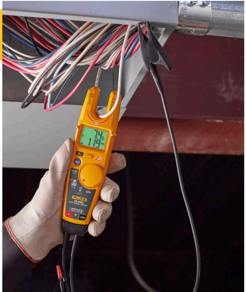
And since the measurement is performed through the cable’s insulation, you reduce exposure to metallic conductors. You also decrease the potential for errors, or making contact with the wrong conductor.
